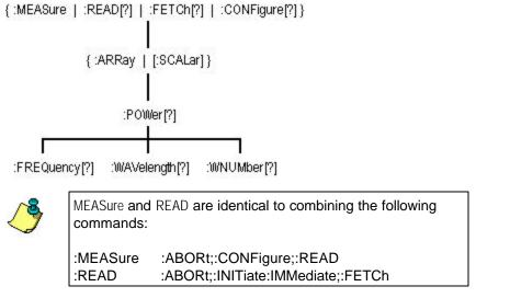
To perform a measurement, add a POWer function to the measurement instruction. The POWer functions select power, frequency, wavelength, or wave number measurements.
